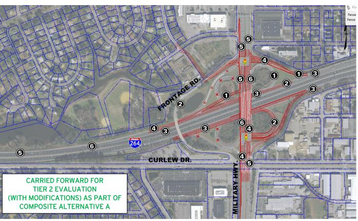
Alternative 2 corrects the deceleration length for the eastbound exit ramp to eastbound and westbound Military Highway, and eliminates merge-weave areas along the I-264 C/D roadways. Traffic operations at the signalized ramp terminal intersections were determined to be acceptable with refinements. Accordingly, Alternative 2 was carried forward for further evaluation in Tier 2 screening.
