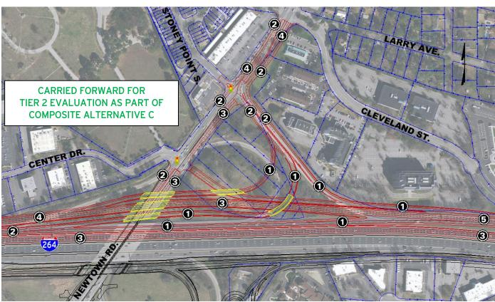
Alternative 4 was carried forward to evaluate the alternative intersection configurations along Newtown Road. Initial analyses indicated favorable intersection operations, with freeway merge-weave operations identical to those of Alternative 3.
