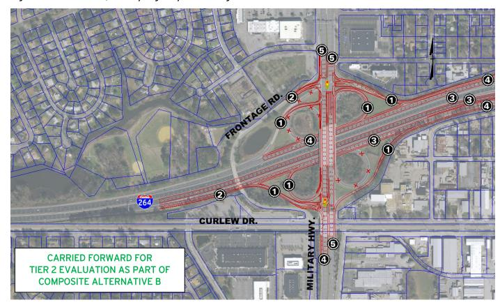
Alternative 1 was carried forward into Tier 2 evaluation based on its ability to eliminate merge-weave areas along the I-264 C/D roadways, and acceptable traffic operations at signalized ramp terminal intersections.
