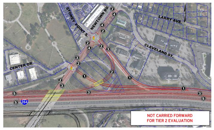
Under Alternative 1, all traffic from Newtown Road enters the westbound I-264 C/D roadway, resulting in heavy downstream weaving movements in advance of the I-264/I-264 interchange. The limited distance between the two interchanges results in poor weave performance. For this reason, Alternative 1 was not carried forward for Tier 2 evaluation.
