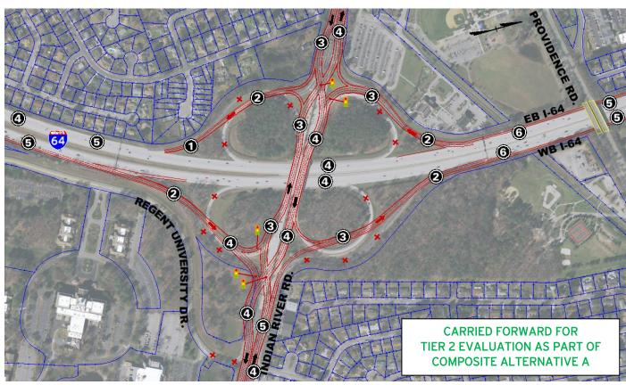
Tier 1 traffic analyses resulted in acceptable levels of service at the crossover intersections along Indian River Road, and eliminates all pedestrian and bicyclist crossings of free-flow ramp terminals. Minor right-of-way impacts were identified. On the basis of these findings, Alternative 2 was carried forward for Tier 2 evaluation.
