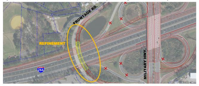
The City of Norfolk requested that the study include evaluation of a signalized right turn movement from the westbound I-264 exit ramp to northbound Military Highway. Accordingly, Alternative 2 at this interchange was also modified to reflect a signal-controlled dual right turn movement at this location, while other alternatives retained a free-flow right turn movement. The signal-controlled movement is shown in Figure 4-26
