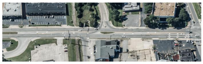
The City of Virginia Beach is reconstructing the roadway between the I-264 overpass and the intersection at Virginia Beach Boulevard to the north. The improvements being made as part of the city's Witchduck Road Phase II improvement project include additional through lanes, additional turn lanes, sidewalks, new traffic signals, and creation of a cul-de-sac on Mac Street with direct access to Witchduck Road eliminated.
