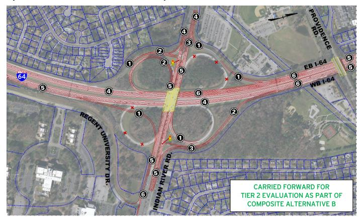
Alternative 1 would provide acceptable traffic operations at signalized ramp terminal intersections, and would eliminate weaving areas on eastbound and westbound I-64. The layout would fit within existing right-of-way. For these reasons, Alternative 1 was carried forward for refinement and further analysis in Tier 2 screening.
