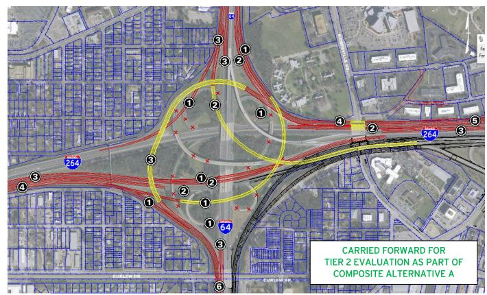
Alternative 3 avoids the use of a fracture-critical viaduct structure in the northwest quadrant of the interchange (as featured in Alternative 2). Left exits and merge weave areas along eastbound and westbound I-264 are eliminated, and operational analyses produced favorable results regarding remaining weave, diverge, and merge areas. Accordingly, Alternative 3 was carried forward for refinement and further evaluation.
