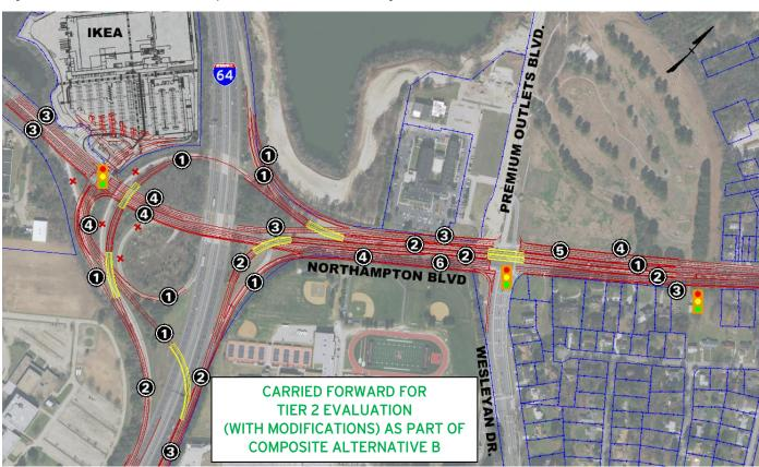
Analyses indicated that Alternative 4 could provide acceptable traffic operations, and accommodate required traffic movements. Like Alternative 2, the number of signalized intersections along Northampton Boulevard is reduced, which would reduce travel delay in the corridor. Alternative 4 was therefore selected for refinement and further evaluation under Tier 2 analysis,
