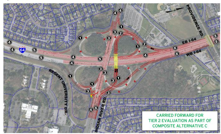
Alternative 3 was advanced for its ability to eliminate weaving areas along eastbound and westbound I-64, and to provide acceptable traffic operations at the new signalized ramp terminal intersection. In addition, the layout requires no additional right-of-way, and reduces the number of free-flow ramp terminals that pedestrians and bicyclists would need to cross. Alternative 3 was advanced into Tier 2 screening.
