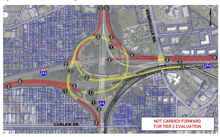
Tier 1 analyses indicates that Alternative 2 would not provide sufficient weave capacity on the westbound I-264 C/D roadway between Newtown Road and I-64. Alternative 2 fails to correct substandard sight distance to the ramp diverge from eastbound I-64 to eastbound and westbound I-264. For these reasons, Alternative 2 was not carried forward for further evaluation.
