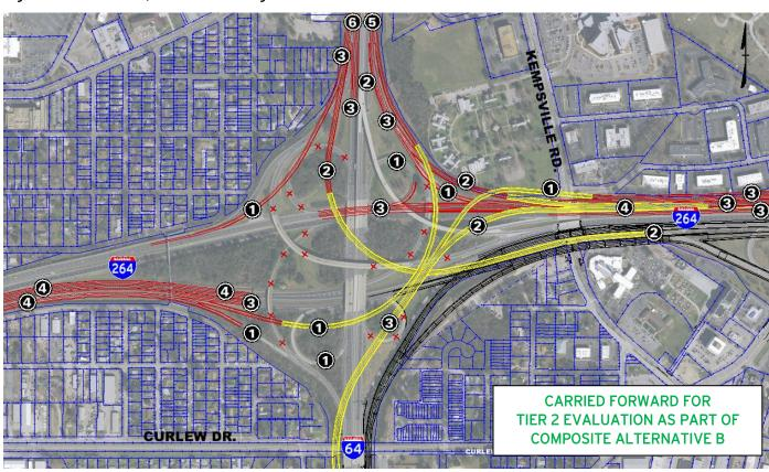
Alternative 4 was carried forward due to its ability to provide full connectivity between both the westbound I-264 mainline and C/D roadways and I-64; elimination of left exit ramps from I-264 and merge-weave areas at closely spaced loop ramps; and favorable results from Tier 1 traffic operations analyses.
