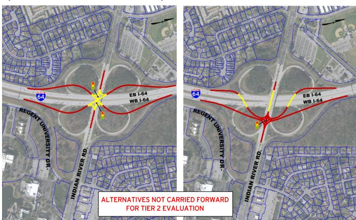
Analyses performed for Alternative 4 determined that a single-point intersection along Indian River Road would operate with heavy delay and a failing overall level of service. The concept is also inconsistent with the Centerville Strategic Growth Area Plan prepared by the City of Virginia Beach. For these reasons, Alternative 4 was not carried forward into Tier 2 screening.
