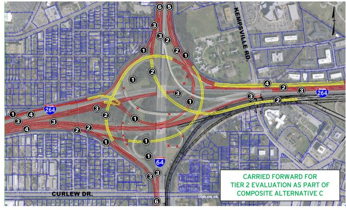
Alternative 5 was carried forward for refinement and further evaluation in Tier 2 screening. Operational analyses indicated favorable results with respect to weave, merge, and diverge conditions, which are different along westbound I-264 than other concepts under consideration. Like other concepts advanced, Alternative 3 eliminates left exits and merge-weave areas at closely spaced loop ramps.
