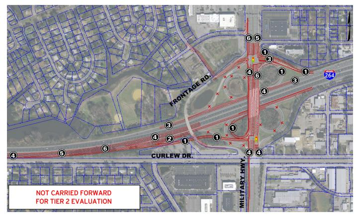
Alternative 3 would introduce an intermediate intersection along the alignment of the exit ramp from the eastbound I-264 C/D roadway. This ramp-intersection arrangement is unconventional, and increases the potential for wrongway entry onto I-264. In addition, the relocated exit ramp from the eastbound I-264 C/D roadway would impact parking spaces at the Tide LRT station. For these reasons, Alternative 3 was not carried forward into Tier 2 analysis.
